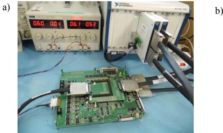
Figure 7. Photo of a) e2v Test Headboard/Controller, b) ESO adaption of the e2v Headboard interfaced to NGC.
