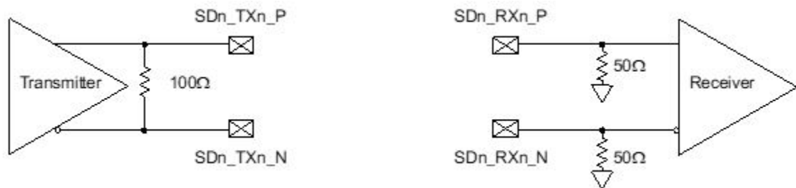
Figure 85. SerDes transmitter and receiver reference circuits
