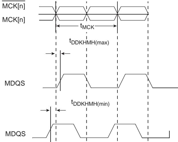
Figure 2-4 shows the DDR SDRAM output timing diagram.
