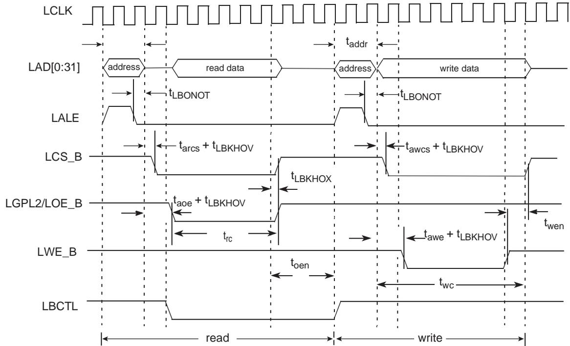
1.  $t_{addr}$  is programmable and determined by LCRR[EADC] and ORx[EAD].
