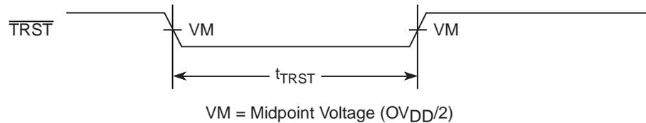
Figure 2-40 provides the boundary-scan timing diagram.
