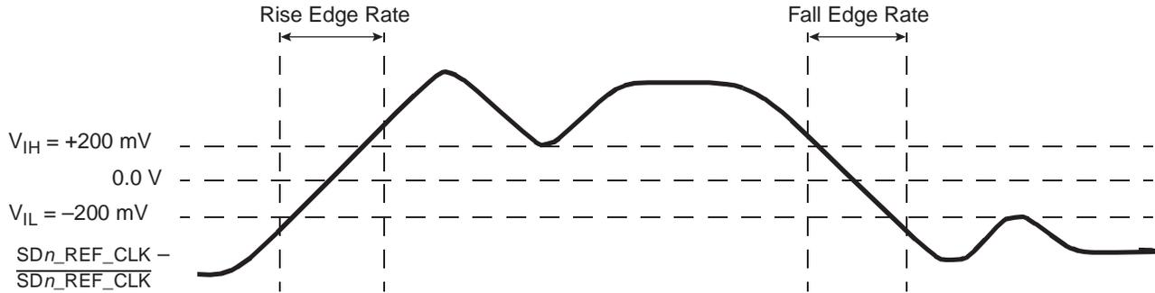
Figure 2-50 shows the single-ended measurement points for rise and fall time matching.
