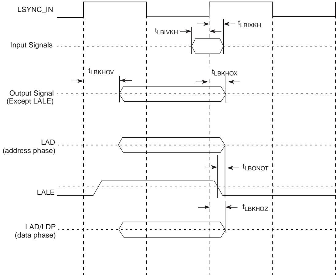
Figure 2-31 applies to all three controllers that eLBC supports: GPCM, UPM, and FCM.
