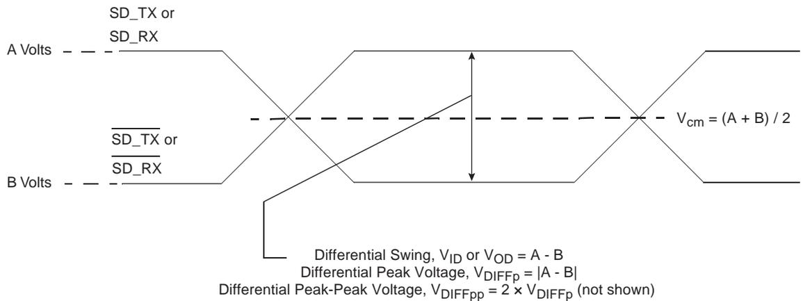
Using this waveform, the definitions are as follows. To simplify the illustration, the following definitions assume that the SerDes transmitter and receiver operate in a fully symmetrical differential signaling environment:
