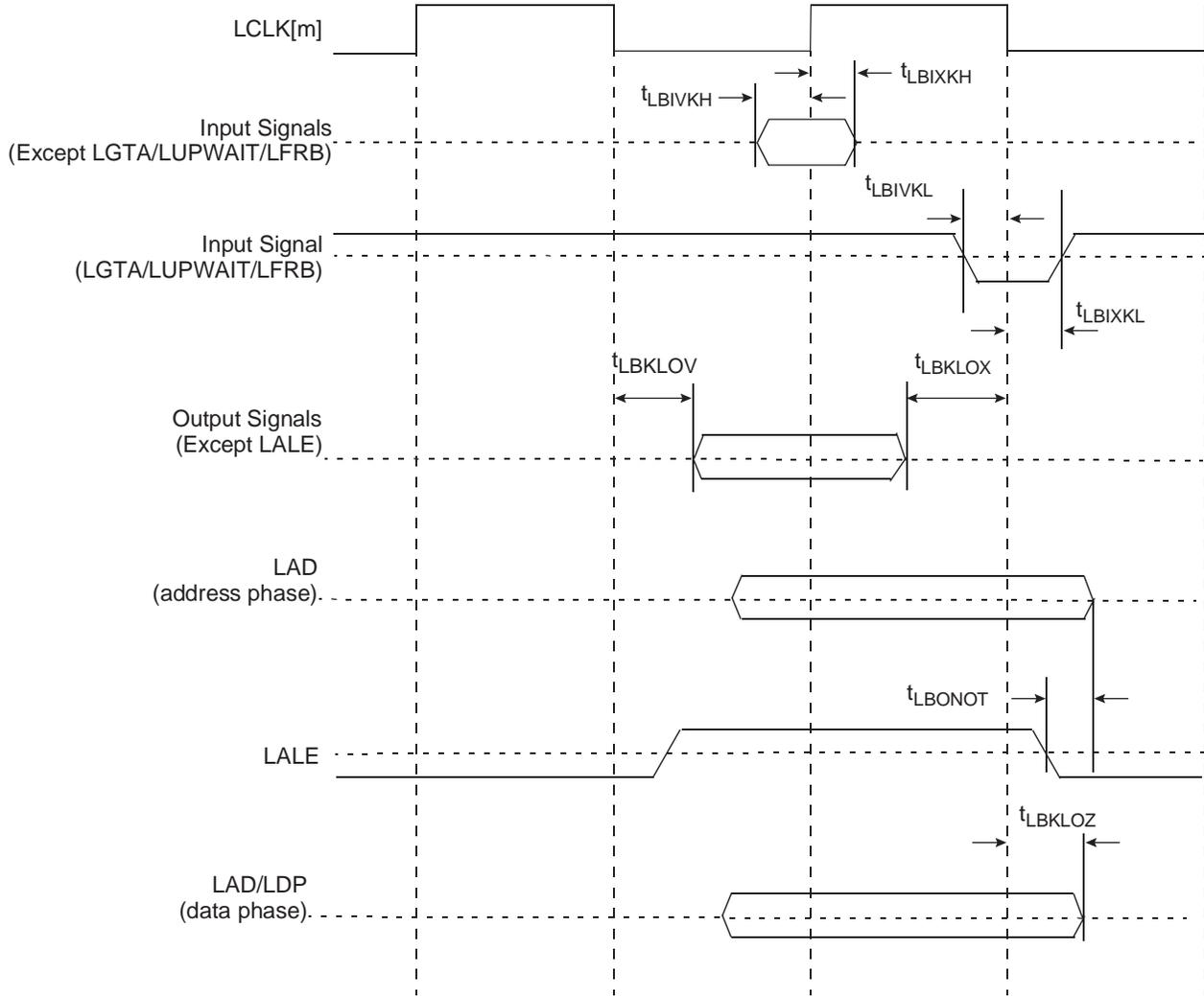
Figure 2-33 applies to all three controllers that eLBC supports: GPCM, UPM, and FCM.
