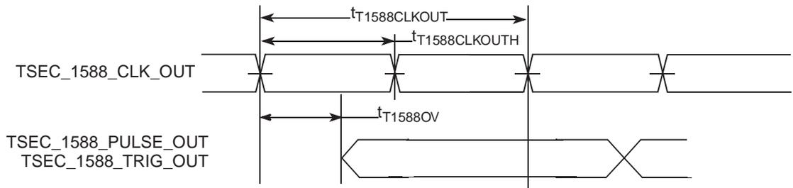
Note: eTSEC IEEE 1588 Output AC timing: The output delay is counted starting at the rising edge if  $t_{T1588CLKOUT}$  is noninverting. Otherwise, it is counted starting at the falling edge.
