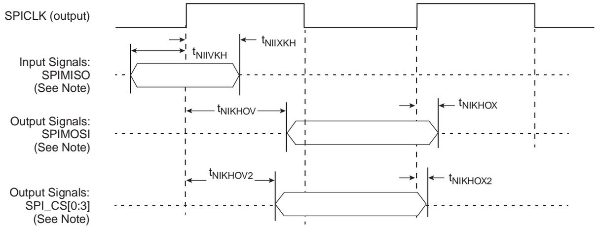
Note: The clock edge is selectable on eSPI.
