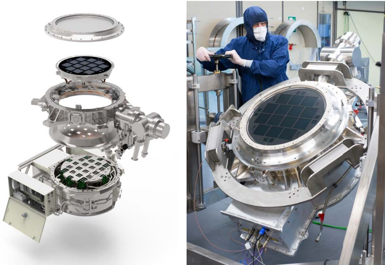
Figure 15. J-PAS Cryocam (a) exploded view (b) photograph of camera
