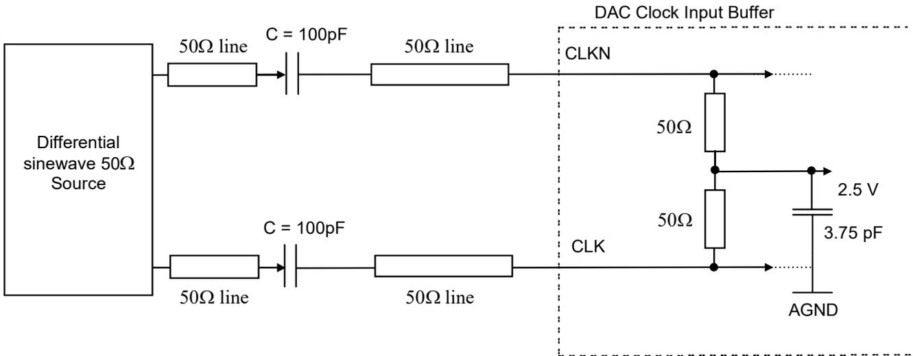
Note: The buffer is internally pre-polarized to 2.5V (buffer between V<sub>CC5</sub> and AGND).
