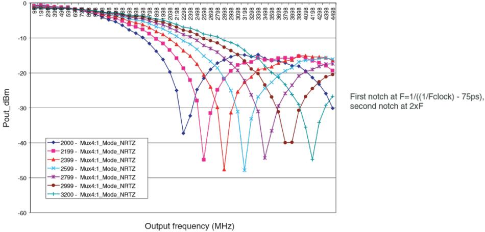
Figure 7-8. Available Pout vs Fout from 98 MHz to 4498 MHz and from 2 Gbps to 3.2 Gbps in RTZ Mode
