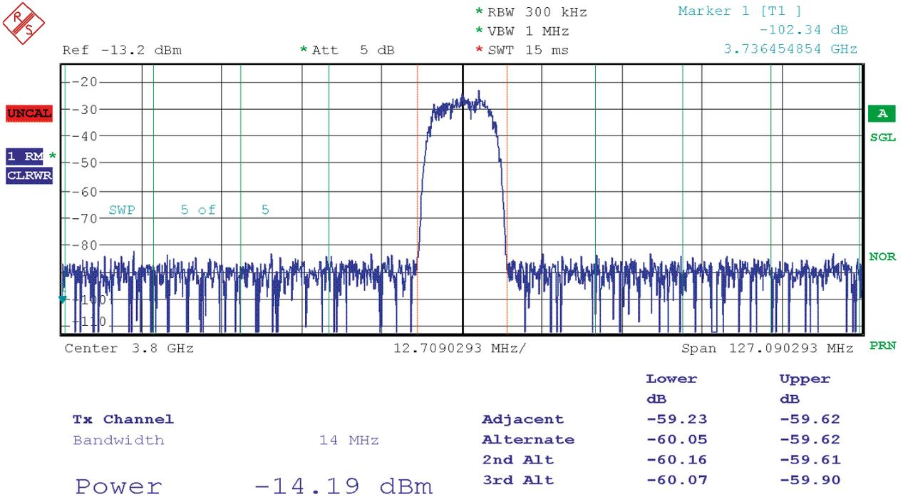
ACPR is in excess of 59 dB. DMWS capability is proven for the third Nyquist zone in RF mode.
