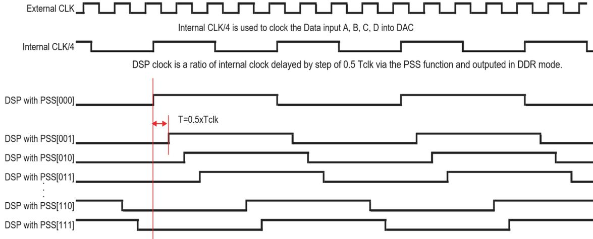
Figure 5-11. PSS Timing Diagram for 2:1 MUX, OCDS[00]
