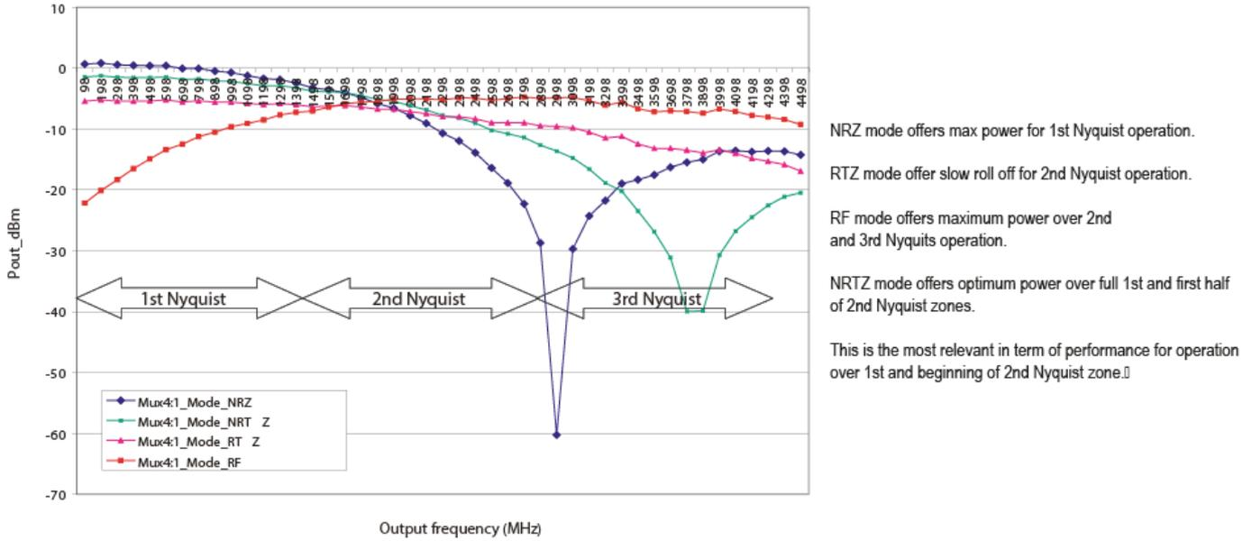
Figure 7-6. Available Pout vs Fout from 98 MHz to 4498 MHz and from 2 Gbps to 3.2 Gbps in NRZ Mode
