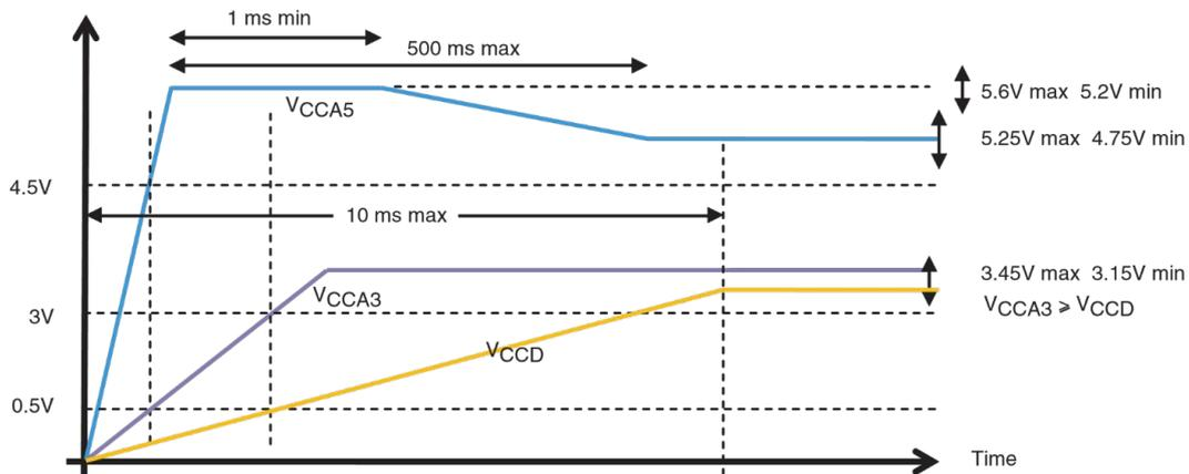
The rise time for any of the power supplies ( $V_{CCA5}$ ,  $V_{CCA3}$  and  $V_{CCD}$ ) shall be  $\leq 10$  ms.
