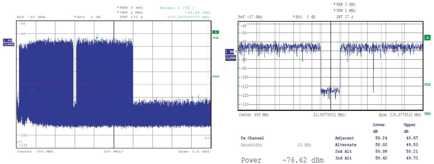
Measured average NPR: 50.02 dB, therefore SNR = 61.02 dB and ENOB = 9.84 bit Effects at low frequency are due to balun and pattern.
