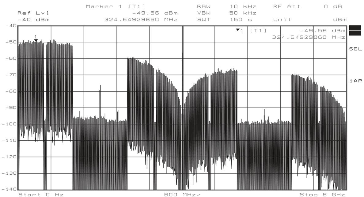
First Zero of the sinc() function is at  $F_{clock}$ .
