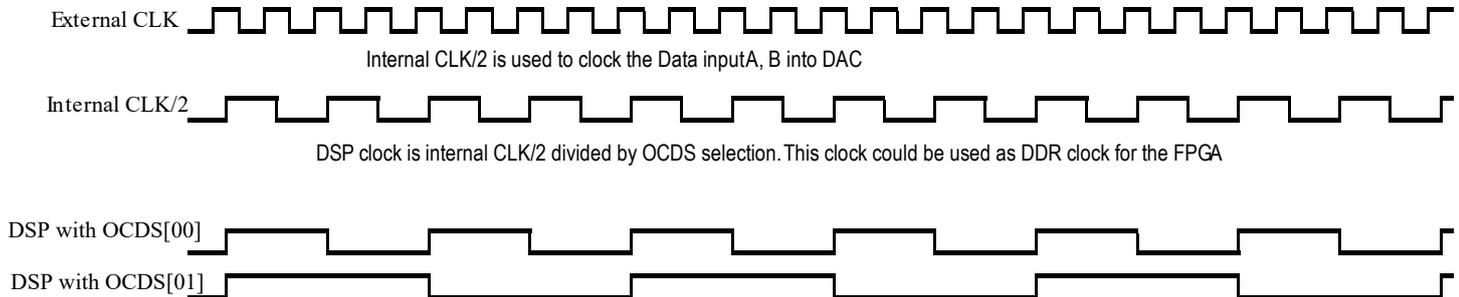
**5.7 Synchronization FPGA-DAC: IDC\_P, IDC\_N, HTVF and STVF Functions IDC\_P, IDC\_N: Input Data check function (LVDS signal).**
