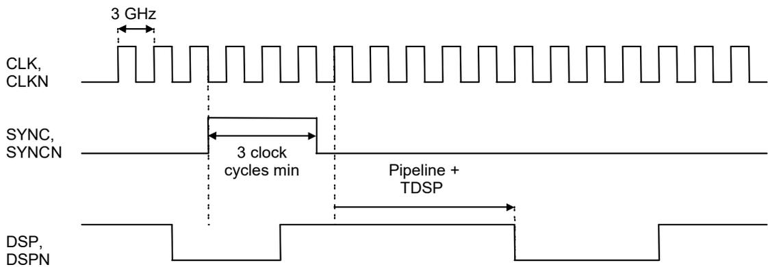
Figure 5-17. Reset Timing Diagram (2:1 MUX)
