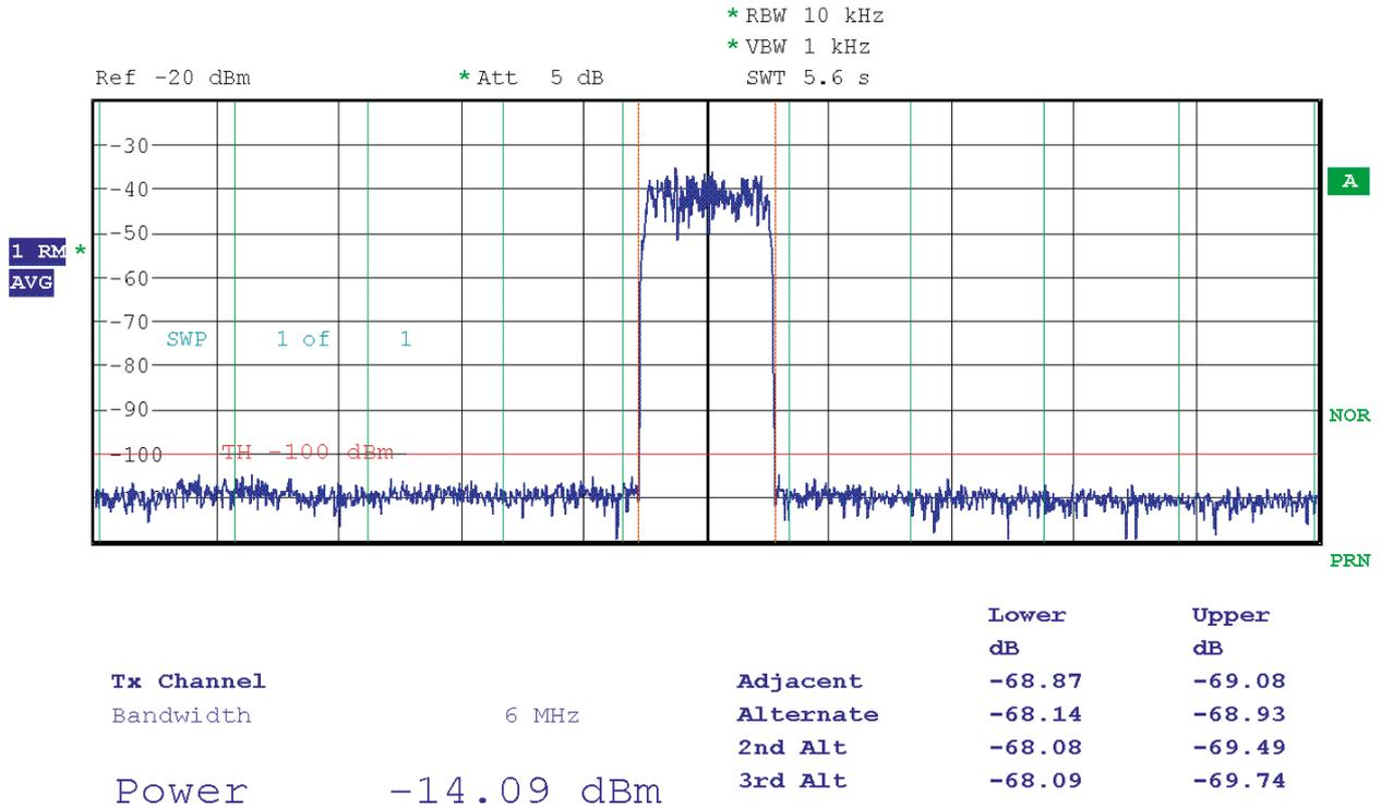
Figure 7-40. ACPR 4 Channels Centered on 900 MHz, Output Mode NRTZ
