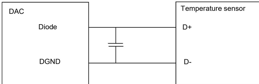
In characterization measurement a current of 1 mA is applied on the DIODE pin. The voltage across the DIODE pin and the DGND pin gives the junction temperature using the intrinsic diode characteristics below [Figure 5-19](#).
