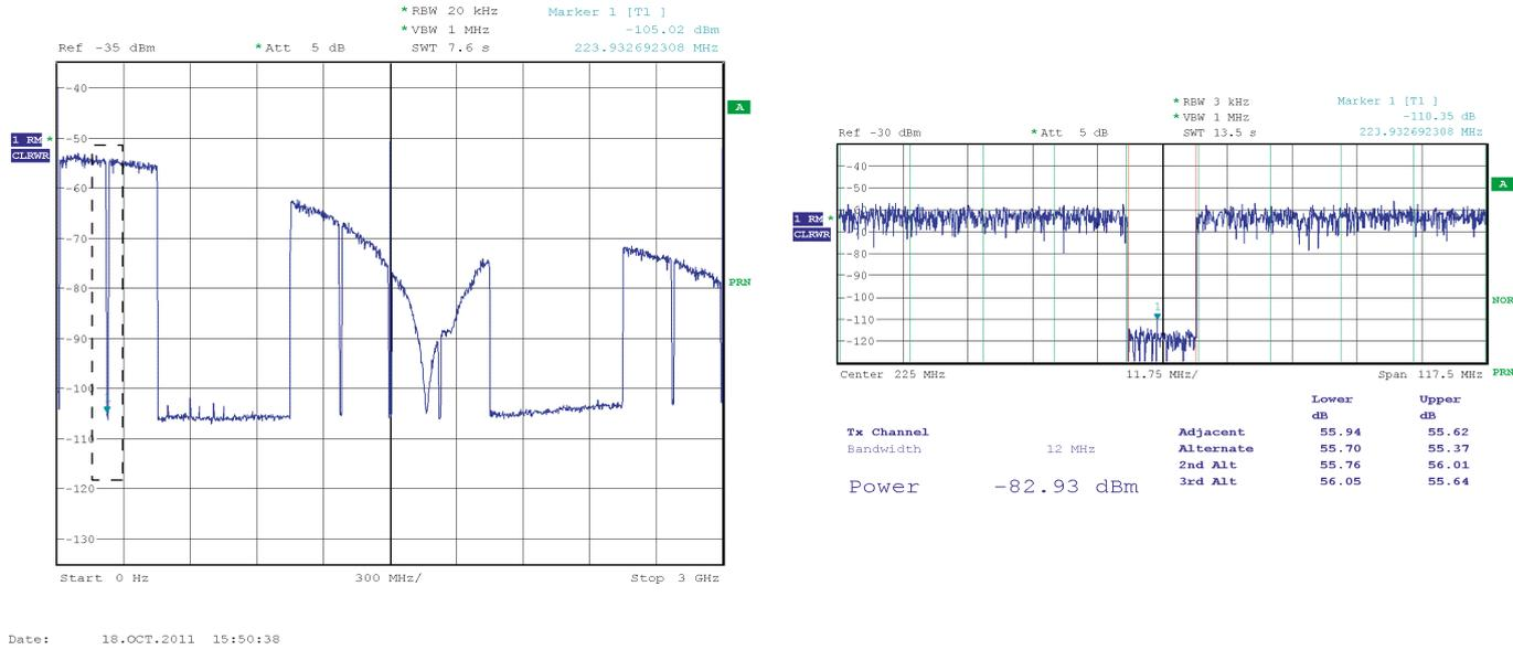
Measured average NPR: 55.7 dB, therefore SNR = 66.7 dB and ENOB = 10.8 bit.
