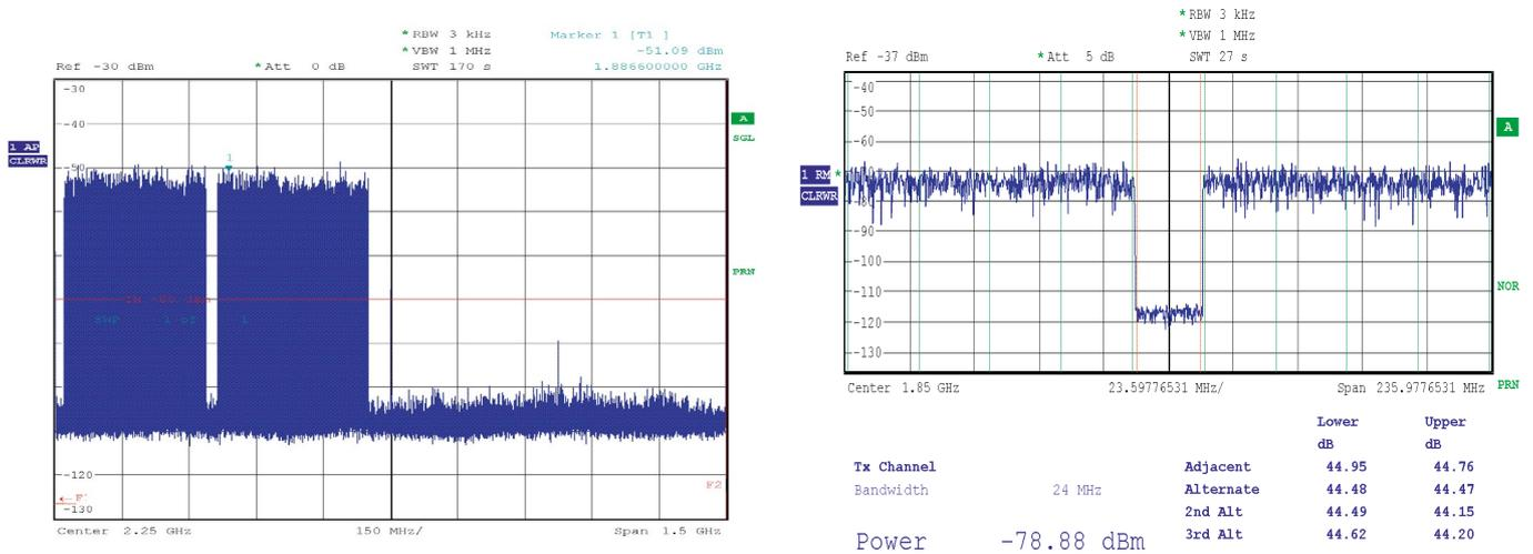
Measured average NPR: 44.6 dB, therefore SNR = 55.6 dB and ENOB = 8.94 bit
