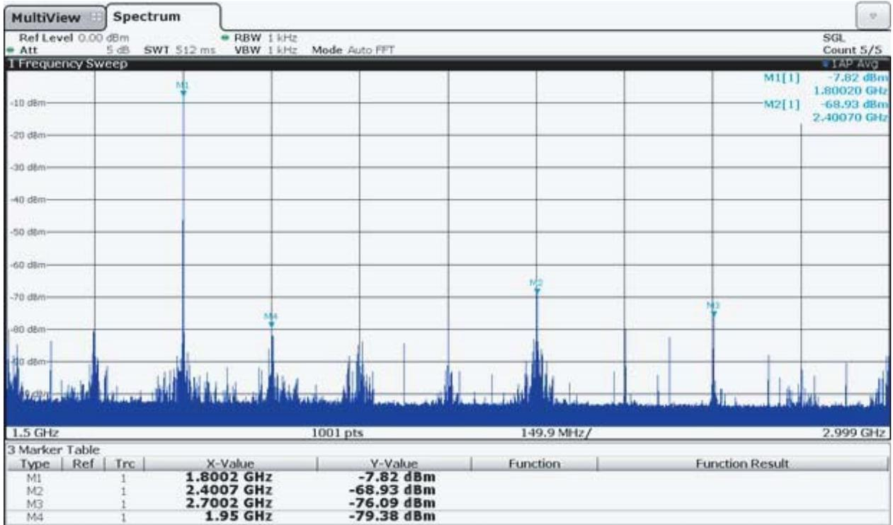
Figure 7-23. Typical SFDR spectrum in RTZ mode. Fout = 2900MHz (2nd Nyquist), MUX4:1, Fs = 3Gps. SFDR = 59dBc.
