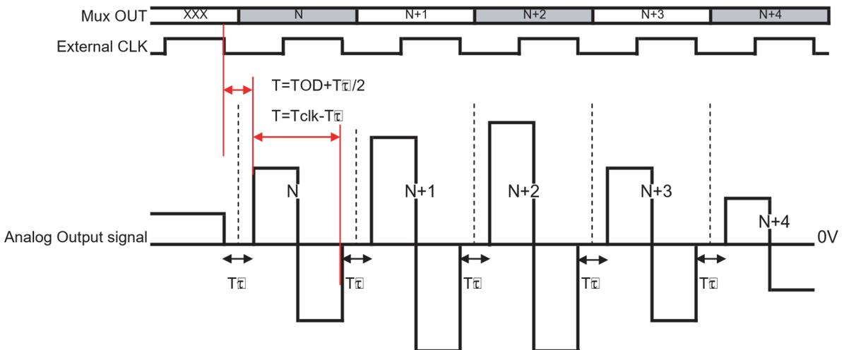
Note: The central transition is not hazardous but its elimination allows to push clock spur to  $2 \cdot Fs$ .  $T_{\tau}$  is independent of  $F_{clock}$ .
