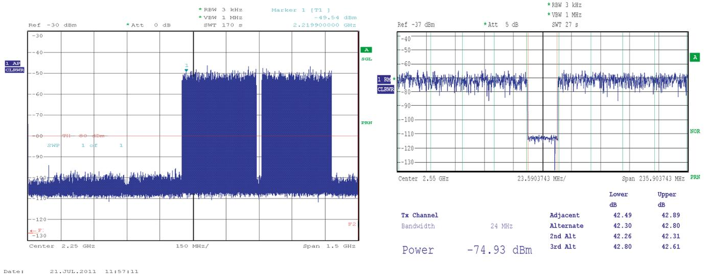
Measured average NPR: 42.56 dB, therefore SNR = 53.56 dB and ENOB = 8.6 bit.
