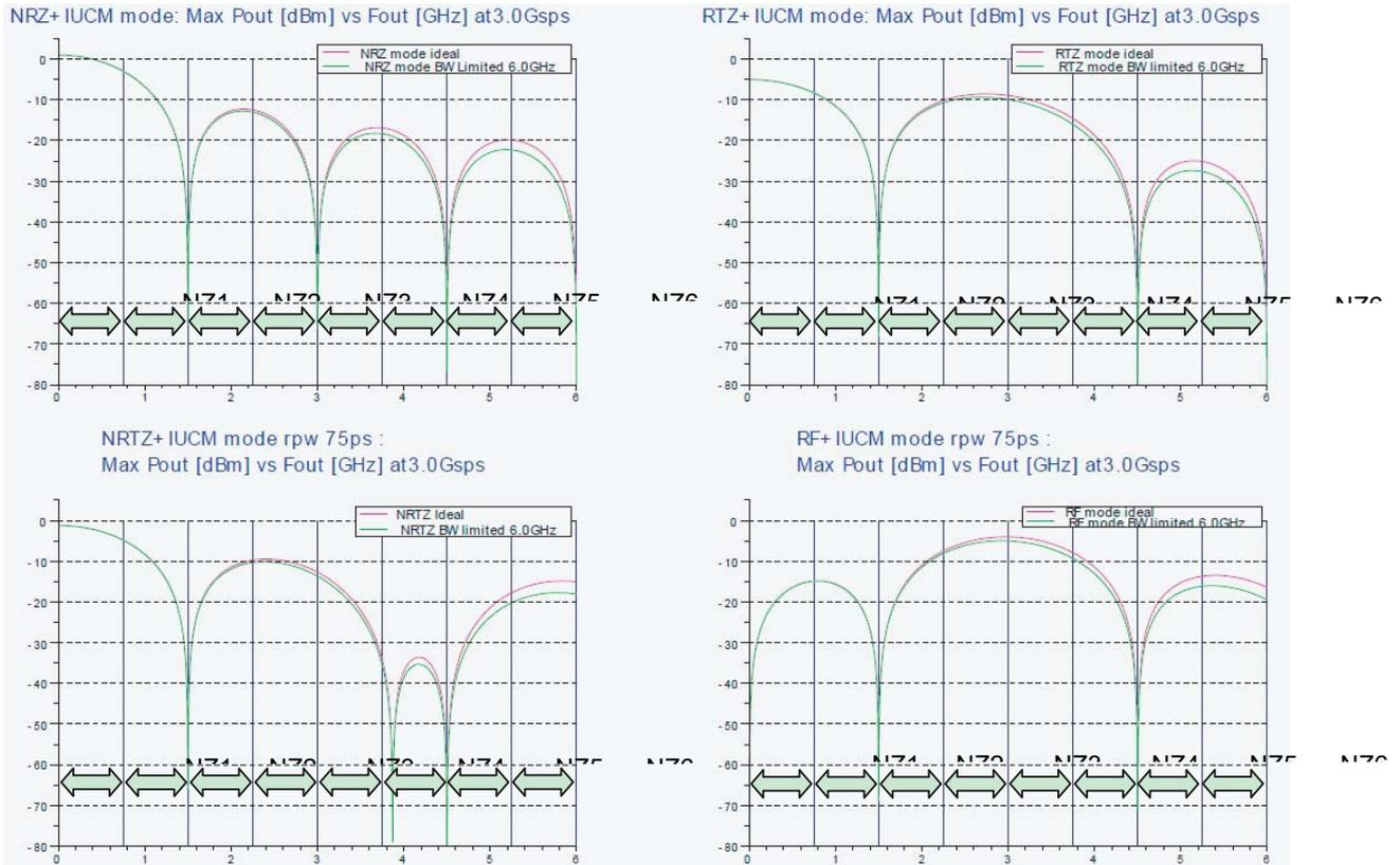
Figure 5-9. Max available Pout[dBm] at nominal gain vs Fout[GHz] in the four output modes at 2 GSps, combined with IUCM, over four nyquist zones, computed for  $\tau\tau = 75$  ps
