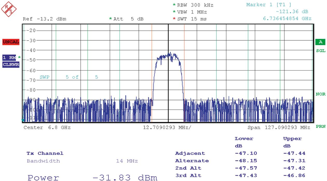
ACPR is still in excess of 47 dB. DMWS capability is proven for the fifth Nyquist zone in NRTZ mode with reduced available dynamic range.
