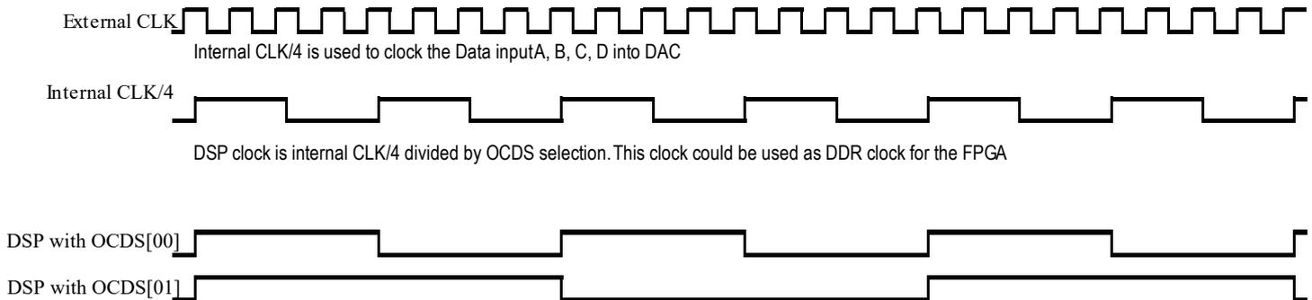
Figure 5-13. OCDS Timing Diagram for 2:1 MUX
