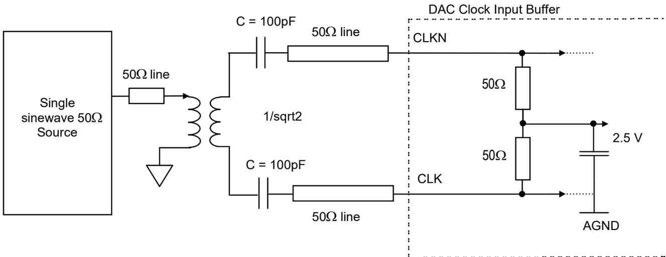
Note: The AC coupling capacitors should be chosen as broadband capacitors with a value depending on the application.
