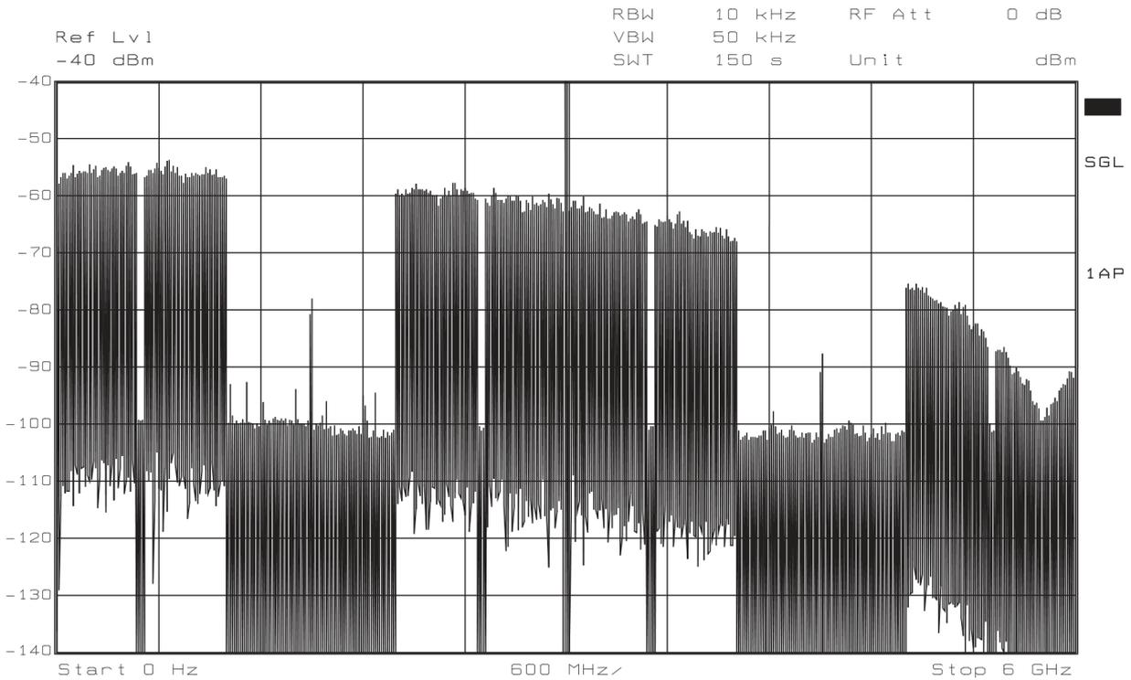
First Zero of the sinc() function is slightly before  $2 \cdot F_{clock}$  which indicates that the duty cycle of RTZ function is a little bit more than 50%, this is due to the balun which introduced some phase error beyond the 180 degrees between CLK and CLKN thus creating a duty cycle on the clock actually seen by the DAC.
