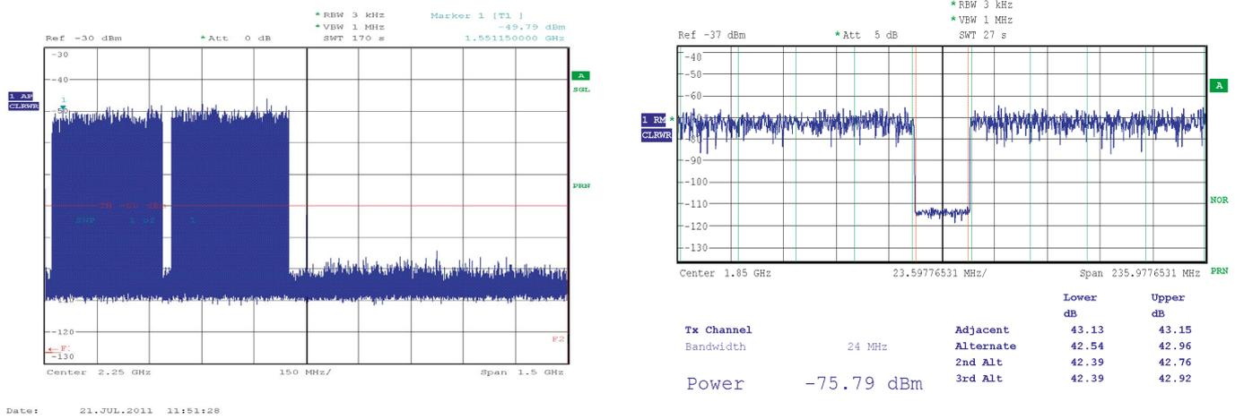
Measured average NPR: 42.78 dB, therefore SNR = 53.78 dB and ENOB = 8.64 bit
