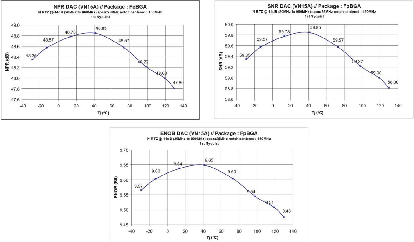
Optimum is at Tj = 40°C, degradation over temp is within 1 dB (or 0.15 effective bit).
