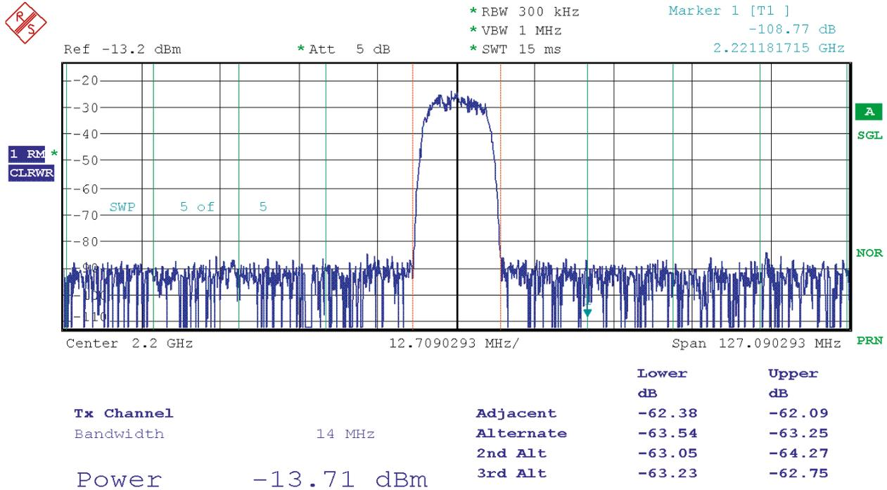
ACPR is in excess of 62 dB. DMWS capability is proven for second Nyquist in NRTZ mode.
