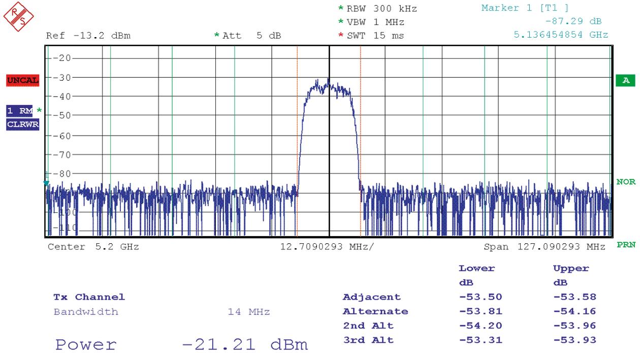
ACPR is in excess of 53 dB. DMWS capability is proven for the fourth Nyquist zone in RF mode.
