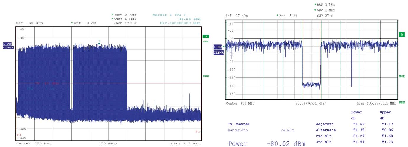
Measured average NPR: 51.36 dB, therefore SNR = 62.36 dB and ENOB = 10.07 bit.
