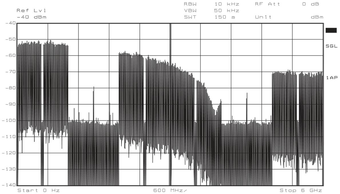
Figure 7-53. Spectrum over 4 Nyquist Zones at 3 Gsps in RTZ Output Mode
