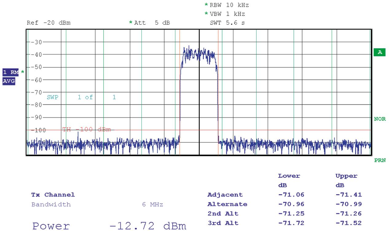
Figure 7-38. ACPR 4 Channels Centered on 300 MHz, Output Mode NRTZ
