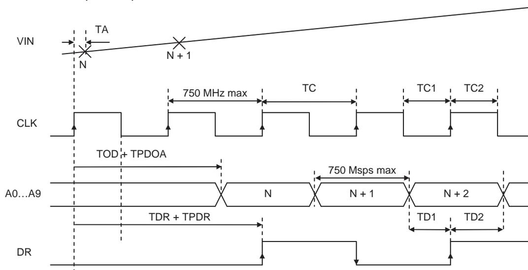
Figure 2-2. Principle of Operation, DMUX 1:2
