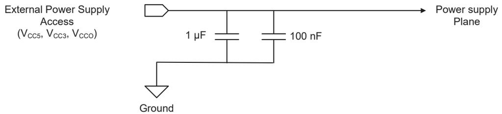
Each group of neighboring power supply pins attributed to the same value should be bypassed with at least one pair of 100 pF in parallel to 10 nF capacitors. These capacitors should be placed as close as possible to the power supply package pins.
