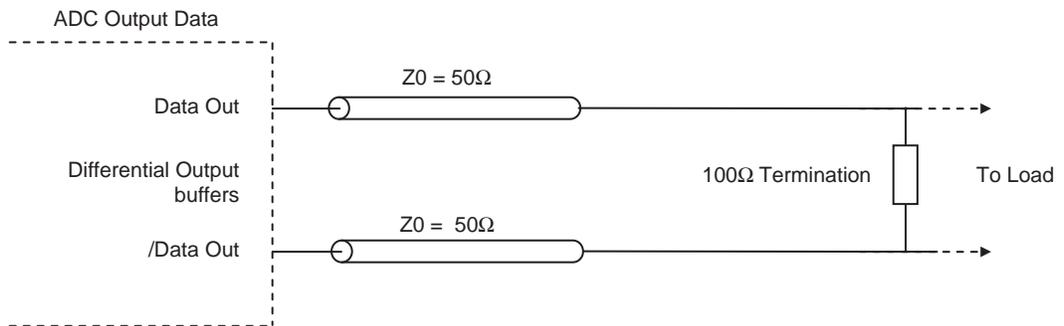
If the ADC is used in 1:1 or 1:2 DMUX modes, the unused ports can be left open (no external termination required).
