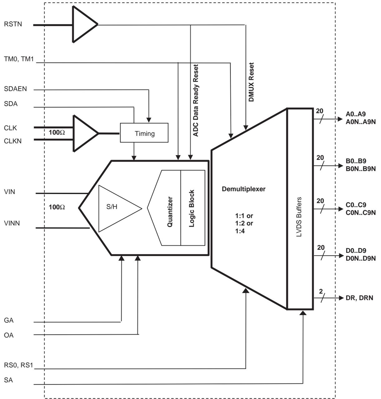
The EV10AS180A is a 10-bit 1.5 GSps ADC. The device includes a front-end Track and Hold stage (T/H), followed by an analog encoding stage (Analog Quantizer) which outputs analog residues resulting from analog quantization. Successive banks of latches regenerate the analog residues into logical levels before entering an error correction circuitry and a resynchronization stage followed by a DEMUX with 100Ω differential output buffers.
