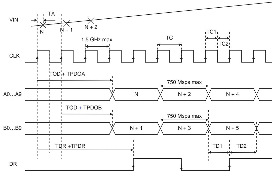
Figure 2-3. Principle of Operation, DMUX 1:4
