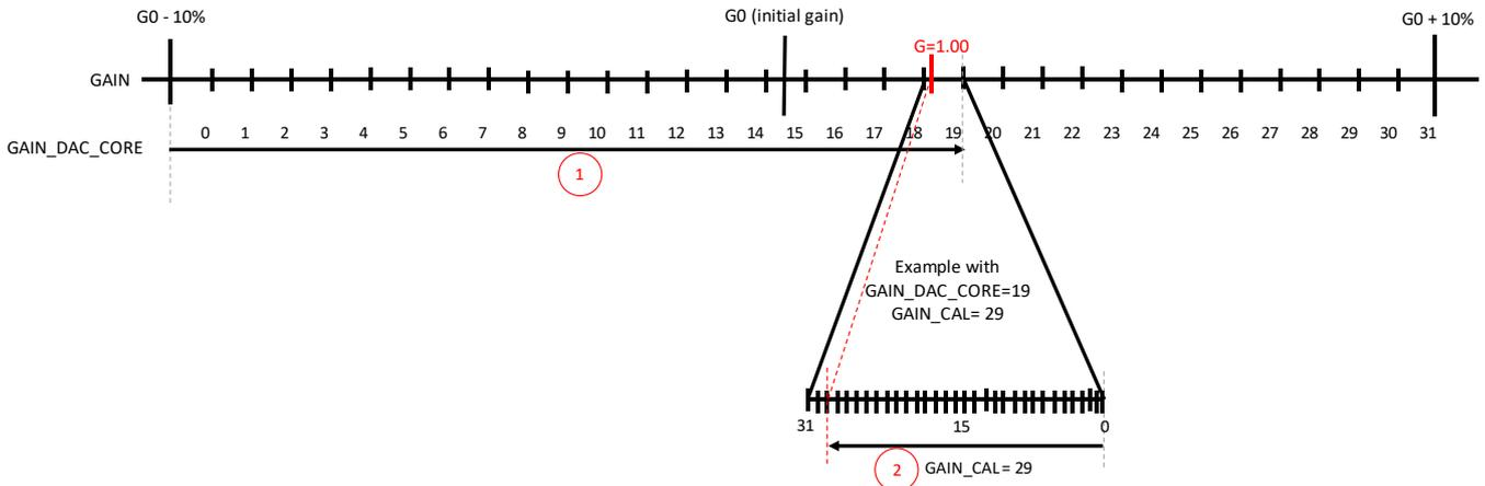
Figure 26: Gain adjustment through  $x\_GAIN\_CAL$  &  $GAIN\_DAC\_CORE$
