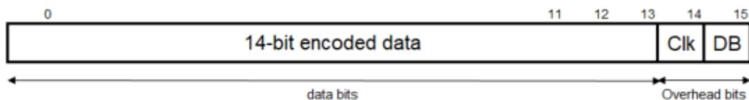
Figure 25: Frame format after encoding
