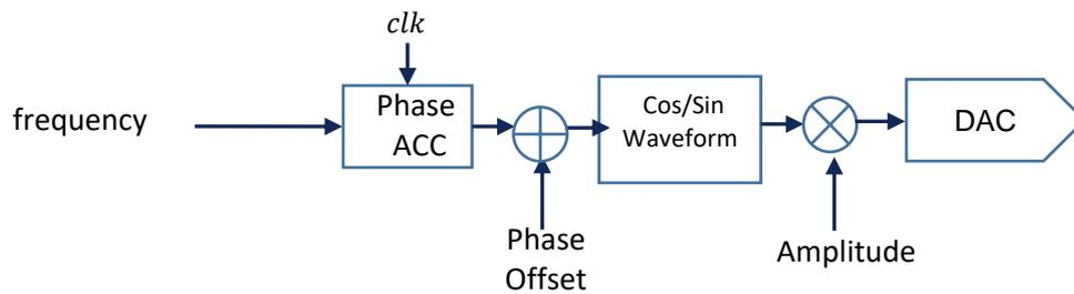
Figure 42 – Direct Digital Synthesis Principle
