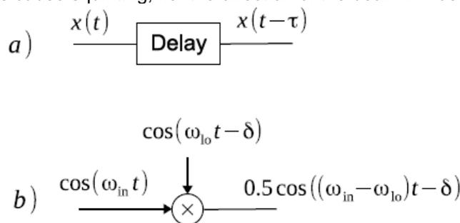
Figure 41 – Time delay a) and phase shifter b)
