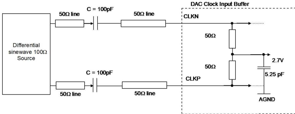
Figure 67: Clock input differential with balun
