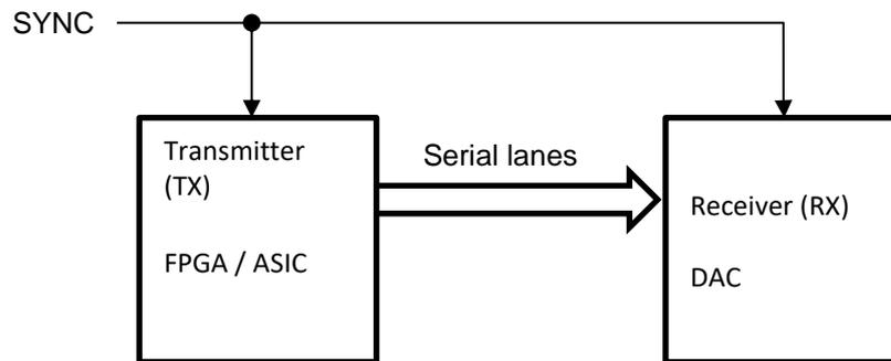
Figure 22: SYNC pulse sequence principle between ESstream transmitter and receiver
