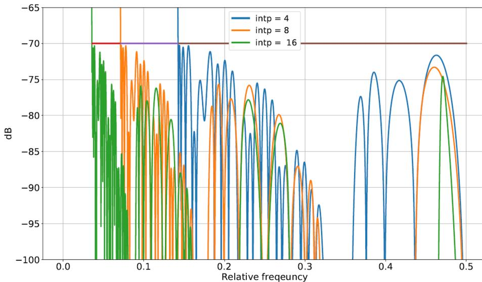
Figure 36 – Interpolation filters, zoom of stopband
