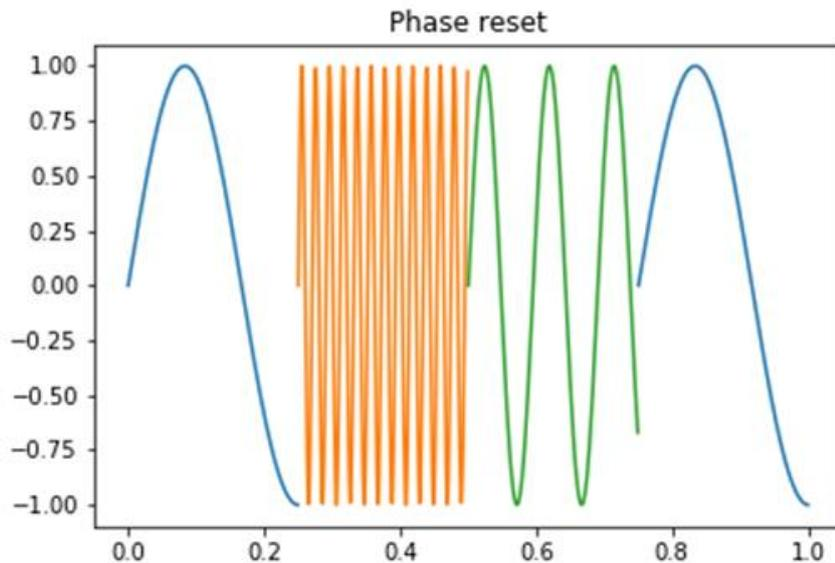
Figure 57 – Example of frequency hopping in phase reset mode
