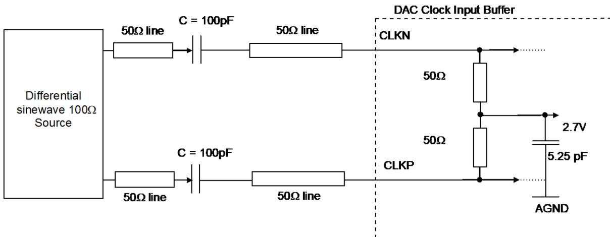
Figure 66: Clock input differential termination
