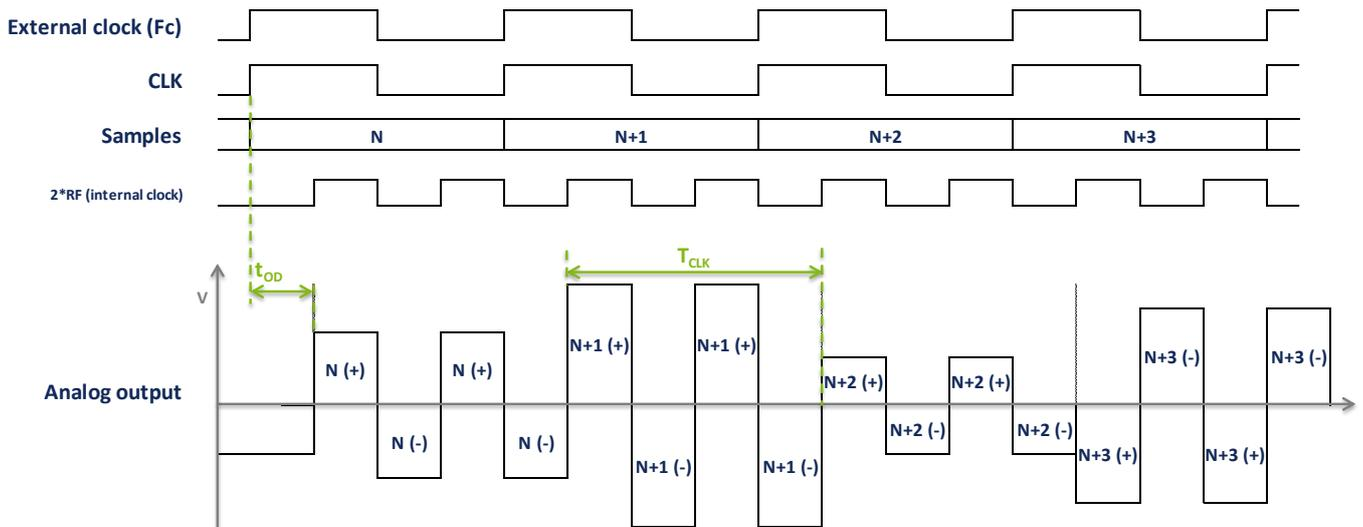
**Figure 30 – 2RF mode timing diagram**
