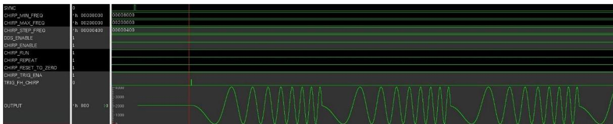
Figure 48 – Chirp mode – Automatic repeat pattern
