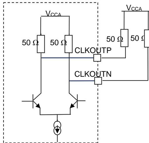
Figure 68: Clock output loading
