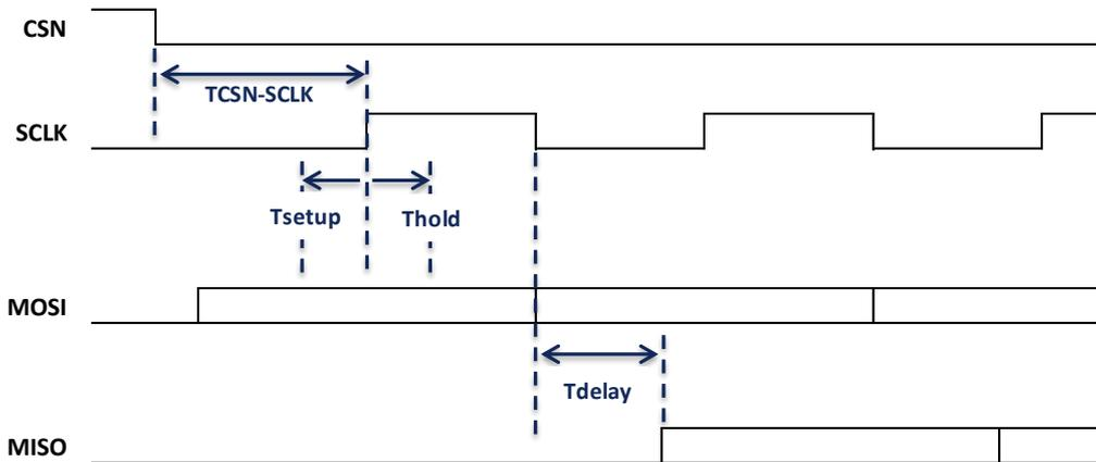
Figure 6 - SPI timing diagram
