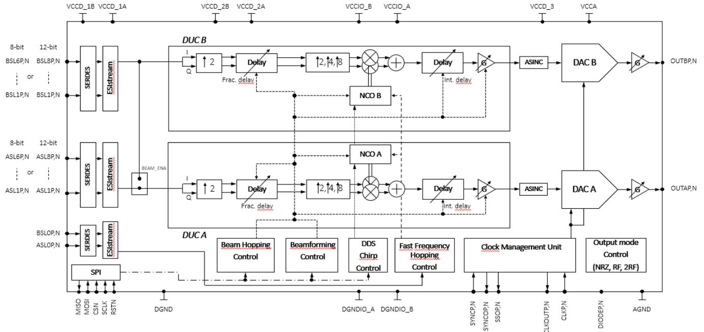
Figure 1: Simplified Block Diagram using Digital Up Converters and Digital features
