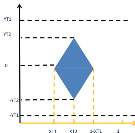
Figure 5 - Serial link eye diagram
