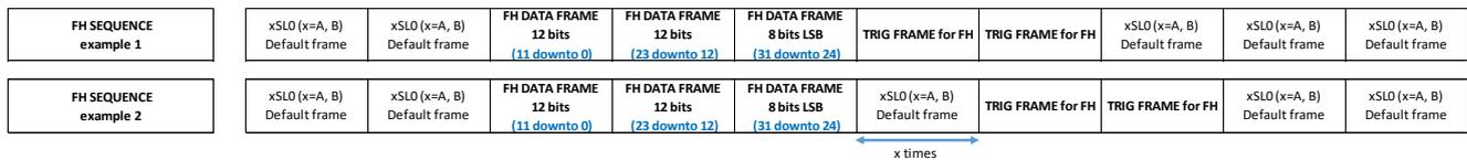
Figure 55 – Examples of frequency hopping programming via xSLO
