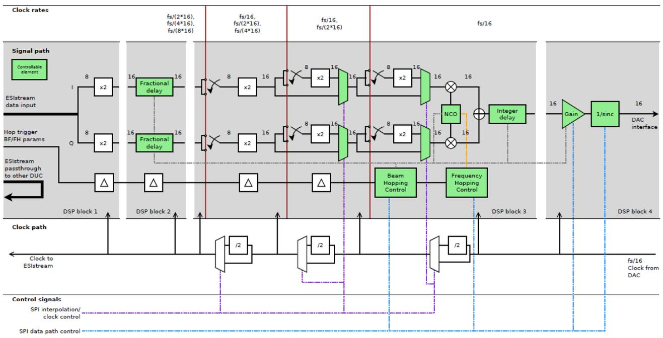
Figure 32 – Signal path with DUC
