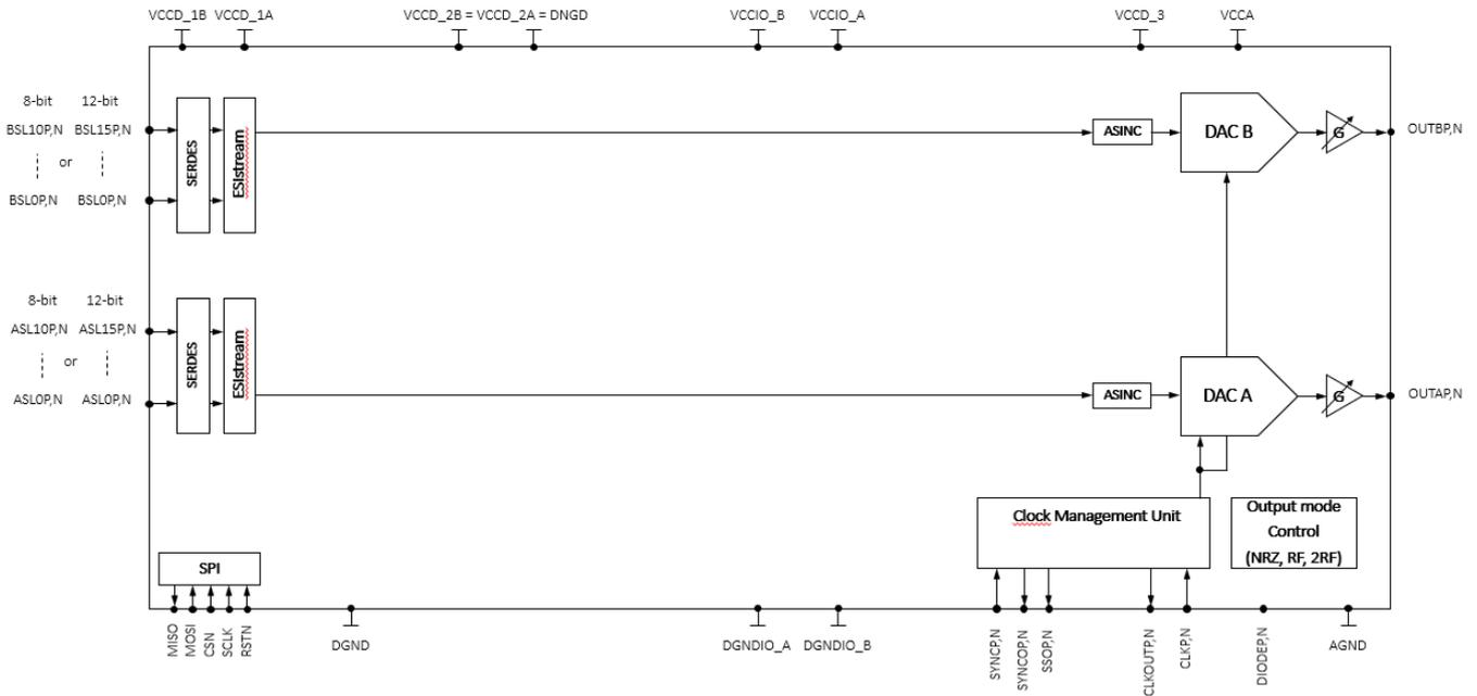
Figure 2: Simplified Block Diagram using Real data
