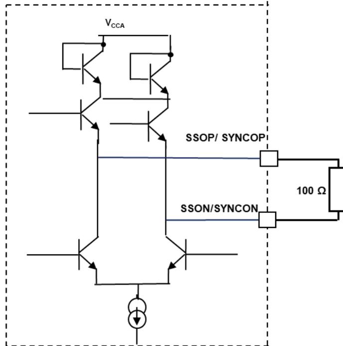
Figure 69: SSO and SYNCO output loading
