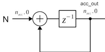
Figure 37 – Phase accumulator
