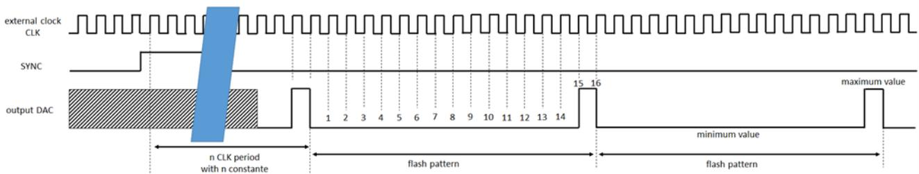
Figure 60: Flash test mode timing diagram
