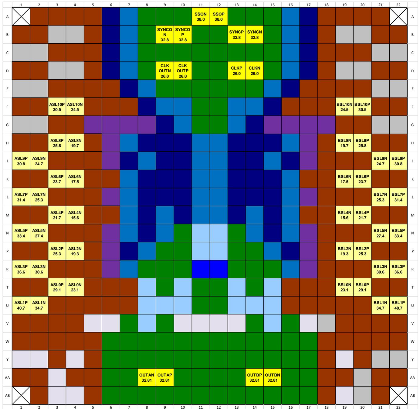
Figure 9 – EV8DD700 relative skews on HSSL, AOUT and Clock signals (values are in ps)
