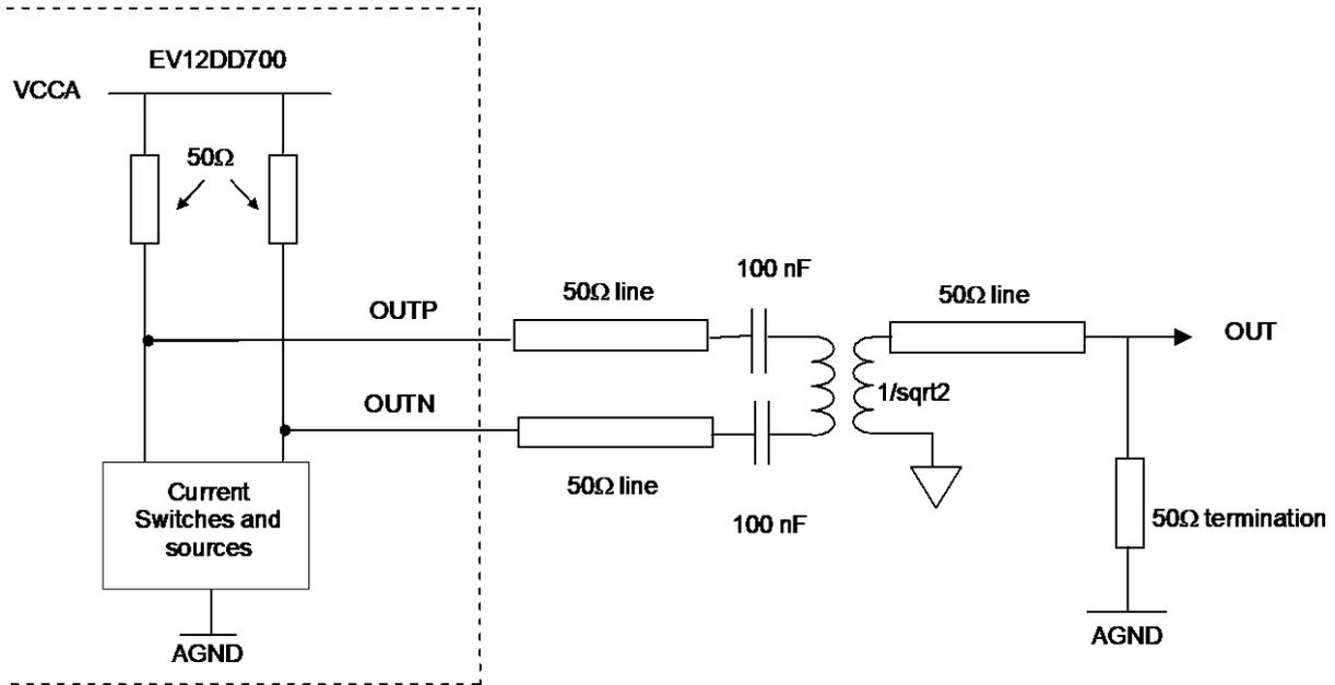
Figure 65: Analog output differential termination using a 1/sqrt(2) Balun
