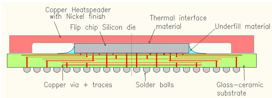
**Figure 12 – Ceramic package cross-section**
