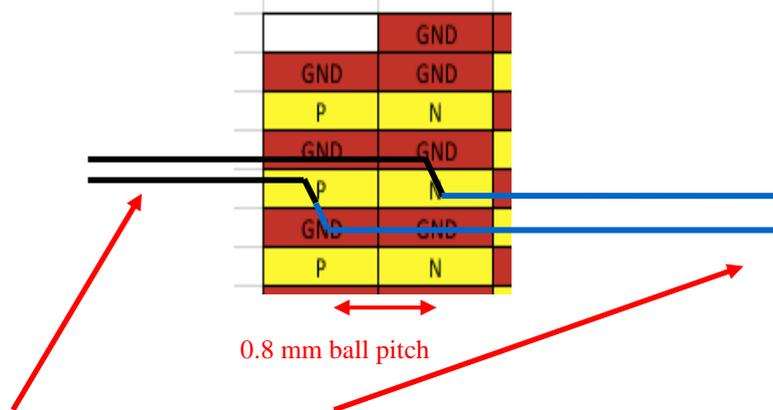
Length on board and length on package are almost the same on N and P (less routing on board for P results from more routing inside package for P).
