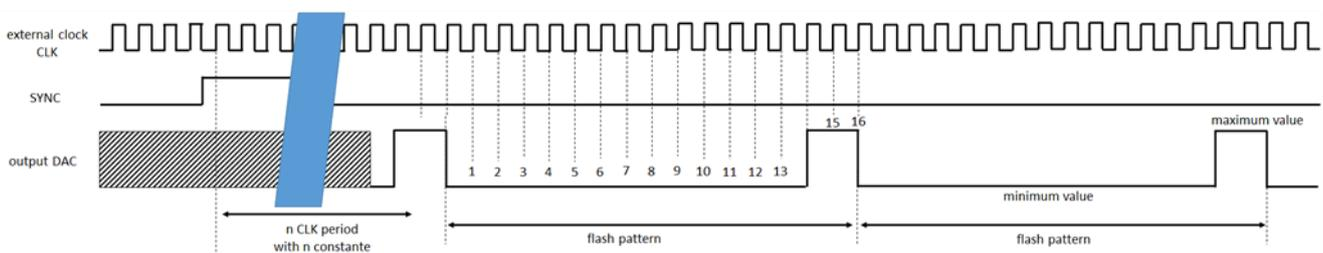
Figure 61: Flash test mode timing diagram (double size maximum value)
