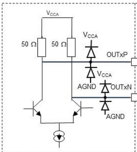
Figure 4: Analog output scheme regarding max ratings
