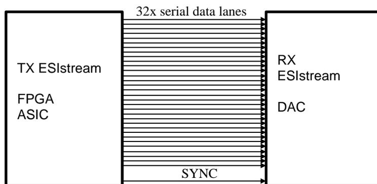
Figure 17: ESistream system example using the DAC
