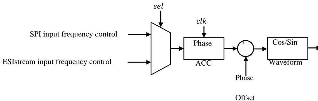
**Figure 49 – Frequency Hopping Principle**
