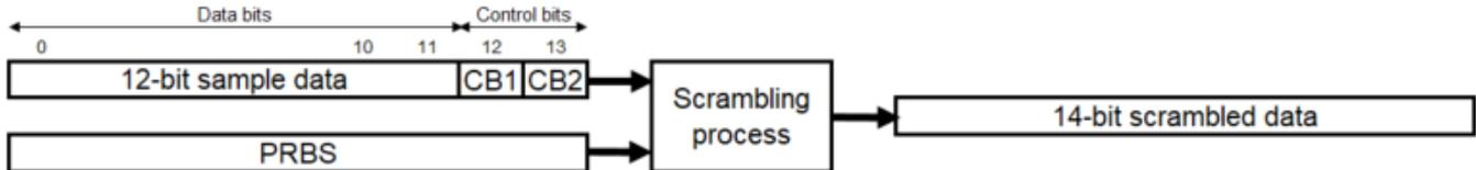
Figure 19: TX 14-bit scrambling process principle
