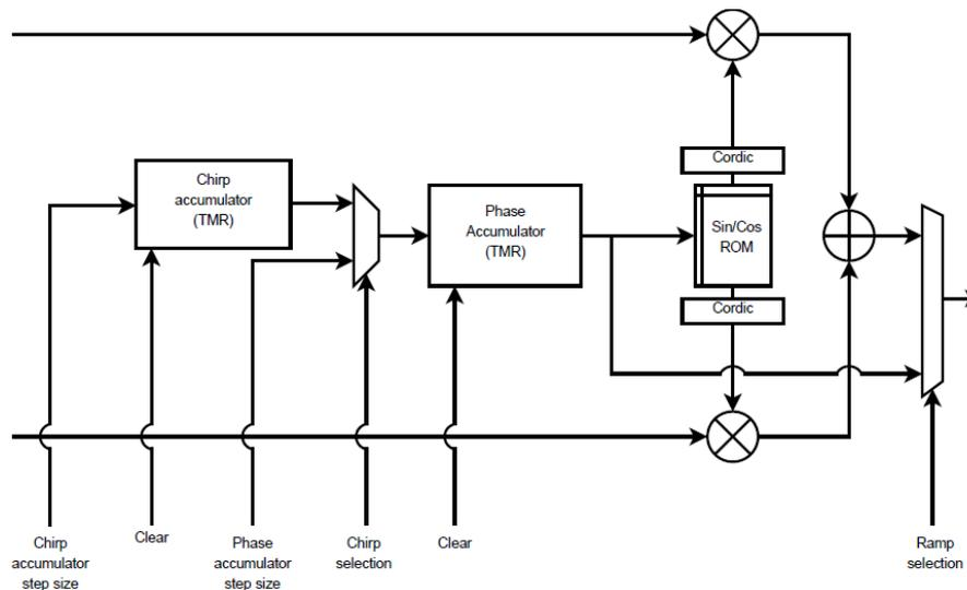
**Figure 45 – Complex mixer configuration for Chirp function**
