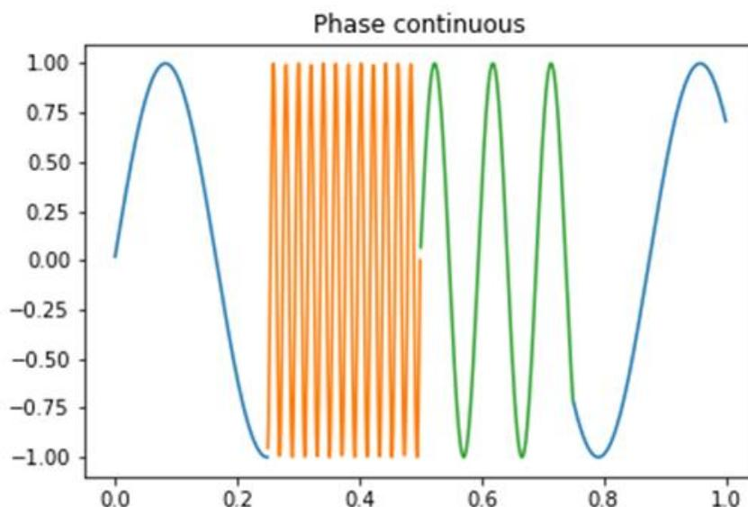
Figure 56 – Example of frequency hopping in phase continuous mode
