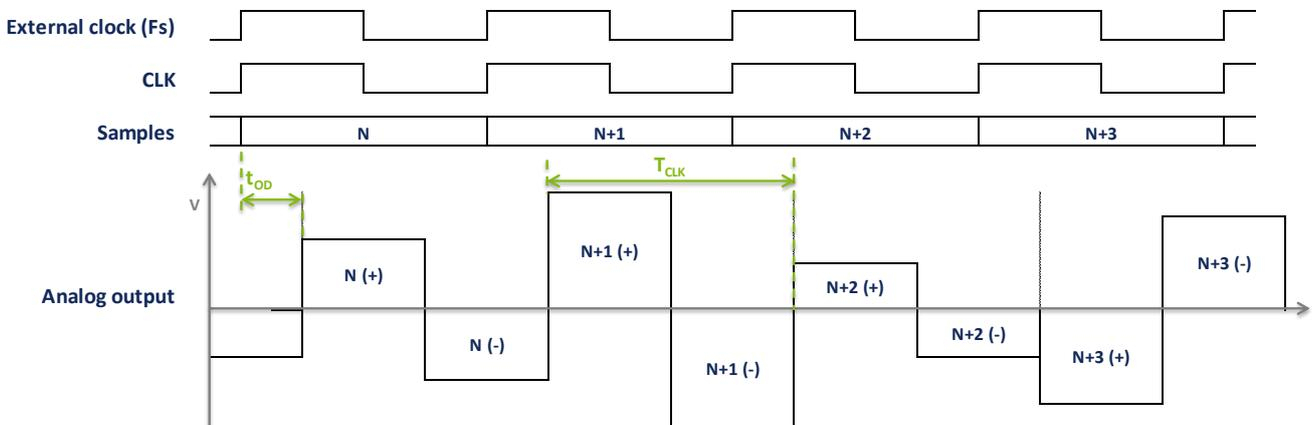
**Figure 29 – RF mode timing diagram**
