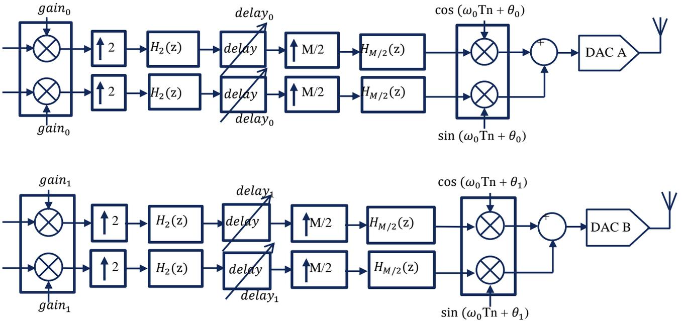
Figure 40 – Beam-forming (Digital Butler Matrix) principle
