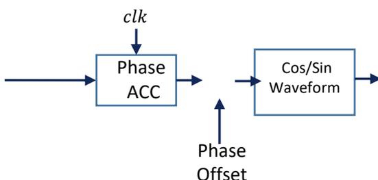
Figure 42 shows a diagram of the programmable complex mixer. In DDS/chirp mode the normal input signal is disconnected and replaced by a constant amplitude.
