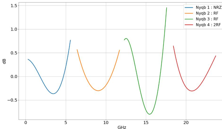
Figure 58 - Remaining error after anti-sinc compensation (Fs = 12 GSps)
