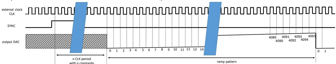
Figure 59: Ramp test mode timing diagram
