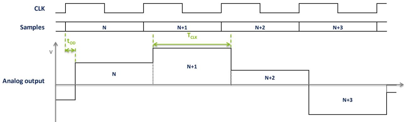
**Figure 28 – NRZ mode timing diagram**
