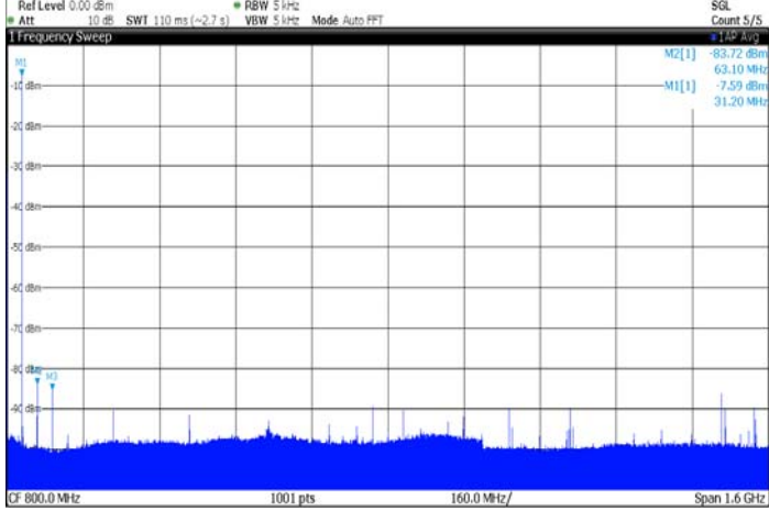
Figure 7-32. Typical SFDR spectrum in NRTZ mode. Fout = 32 MHz (1st Nyquist), MUX2:1, Fs = 3.2 GSps. SFDR = 76 dBc
